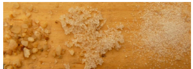
Figure 7: Coarse (16 grit), Medium (36 grit), Fine (60 grit) SiO 2
