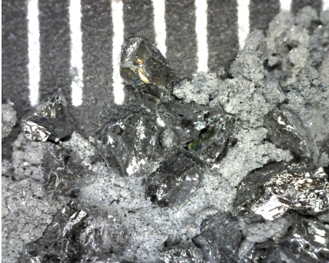
Figure 20: Shattered and undamaged SiC, J7 – 50X
