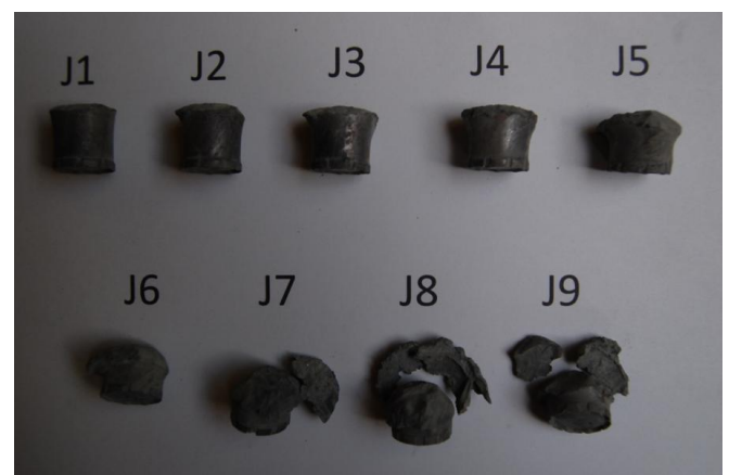
Figure 17: Test J – Steel penetrator condition
