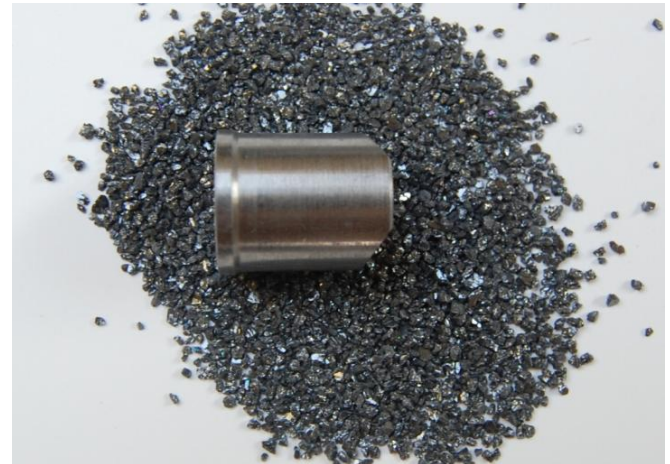
Figure 15: Coarse (16 Grit) Silicon Carbide (SiC) with 20mm steel FSP
