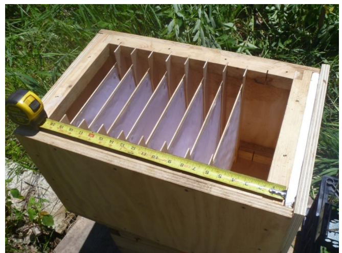
Figure 3: Test box with paper witness panels
